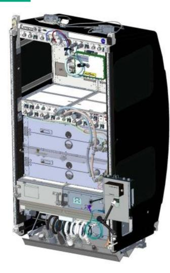
Hardware: HPE Edgeline EL4000 (edge-focused single socket with a single GPU)
